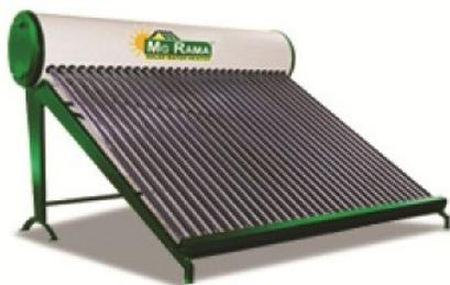
MG Rama Energy offers Evacuated Tube Based Solar Water Heating system for your hot water usage. There are two glass tubes which make single evacuated vacuum glass tube. The tubes are fused on one side and hermetically sealed with each other on the other side. The internal glass tube is coated with highly observing environmental friendly coating to trap the solar energy. The sunlight radiation falls on the glass tube passes
